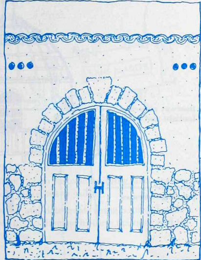
Example 2. Basic wall construction coral rock and stucco; (a) coral rock voussoirs/keystone, (b) barrel tile roof; (c) clay vents (d) double -leafed wooden doors with turned wooden spindles
