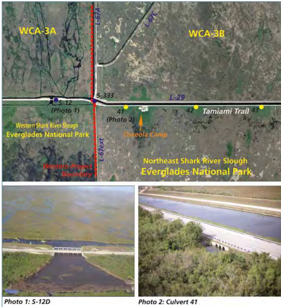
Figure 7. Significant differences exist between the sections of Tamiami Trail corresponding to Western Shark River Slough (west of the project area boundary or S-333) and the road corridor within the project area (east of S-333). When compartmentalization of Water Conservation Area (WCA) 3 was completed in the 1960s, the western section of Tamiami Trail was raised and the high-capacity S-12 water control structures were added to allow increased flow capacity to Western Shark River Slough (see Photo 1). In contrast, the portion of Tamiami Trail east of S-333 was not raised and has retained the culvert design until now. This eastern portion corresponds to the project area (see Photo 2).
