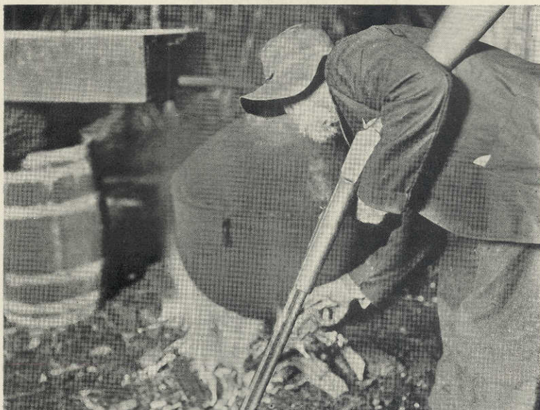
The cover, deftly fashioned from a huge cypress stump, converts the kettle into a retort.
