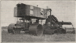
The same ditcher as that shown in the illustration above, after the cabin had been mounted in place
