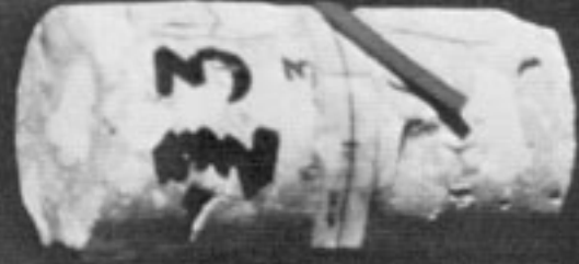
INITIAL COMPRESSION FAILURE VERTICAL CRACKING
