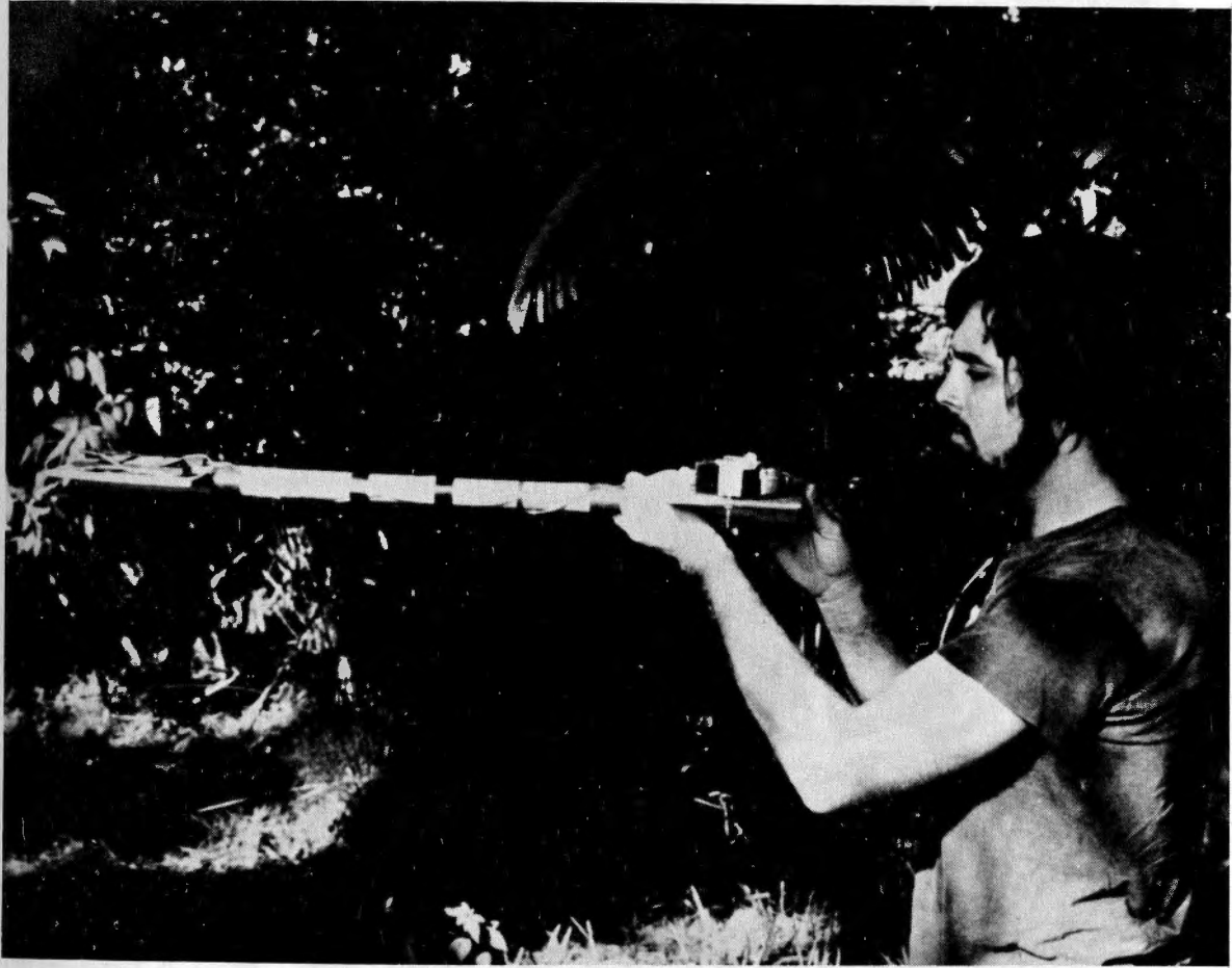
Figure 7 Taking a Light Reading with Photocells
