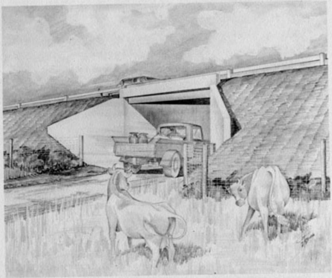
Figure 7. Typical Farm Road Crossing
